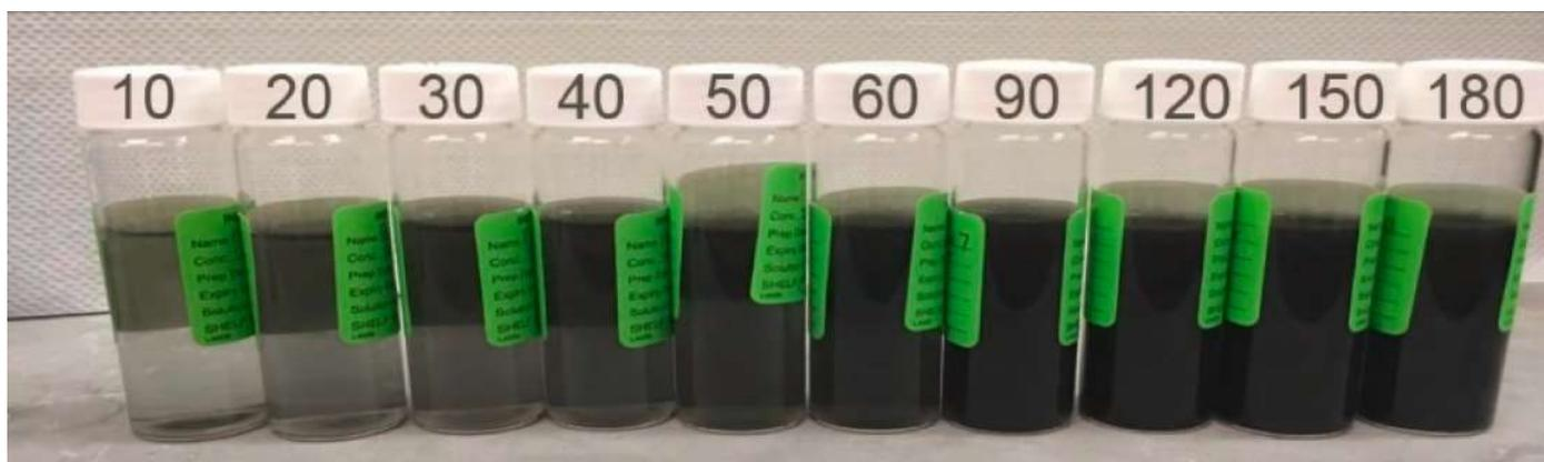
**Figure 1** - PetroFix concentrations in 40 mL VOA vials. If a vial can be seen through (<100 mg/L) it is safe to sample and send to the lab.
